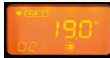
First alarm (orange)
